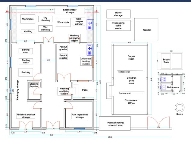
Figure 5. Bonbon Bouye plant floor plan (approx. 25 x 14 meters).<sup>1</sup>
