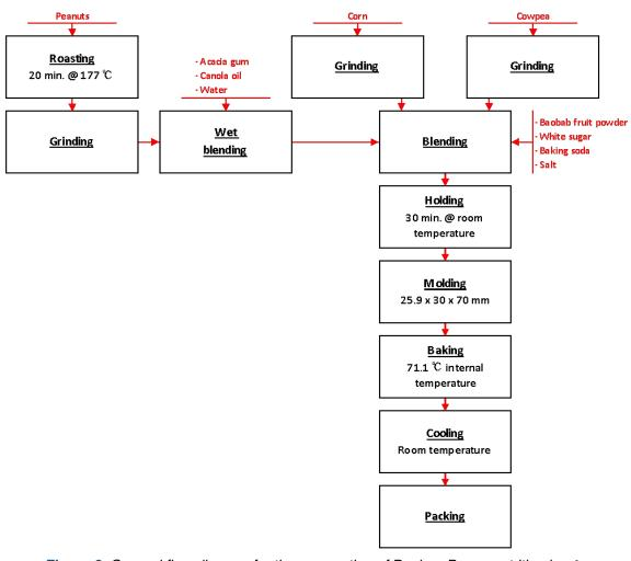
Figure 3. General flow diagram for the preparation of Bonbon Bouye nutrition bar.6
