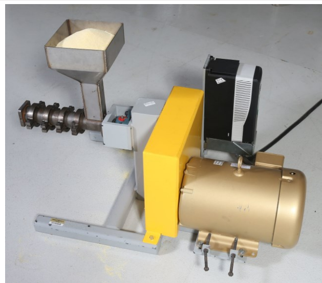
Figure 1. Purdue University's small extruder. (Photo courtesy of Purdue University [Purdue Agricultural Communication/Tom Campbell])
